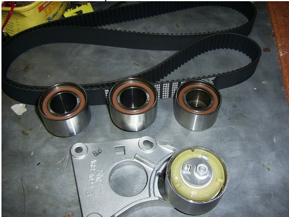
Cambelt Kit. That square hole is where the 1/2" drive T-Bar fits.
